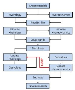
After the model are chosen and coupling settings are defined in the GLOFRIM ini-file, the ini-file is read by GLOFRIM to first initialize the model-specific configuration files and then initialize both models as a coupled entity.
